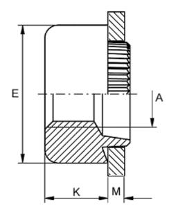
Female thread A = M14Height K = 10.0Outer diameter E = 25.0Plate thickness = 2.6 to 2.8
